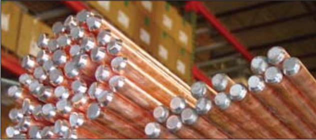
these non-compliant diameter rods that the market was forced to offer either a full 5/8 inch (0.625) diameter rod or a ground rod that is listed by a certification agency.
